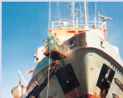
Spot repair and surface preparation of ship hulls with the 3000-bar Modular Gun System .
