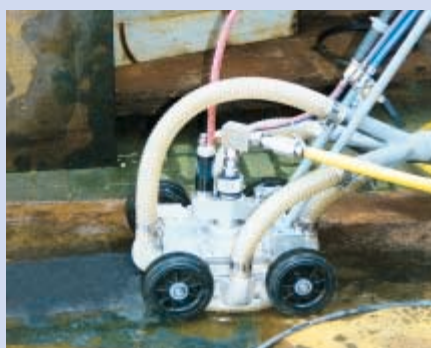
Emission-free deck cleaning, paint stripping and surface preparation with the 2500-bar jetting tool Vacu Jet 2500 .
