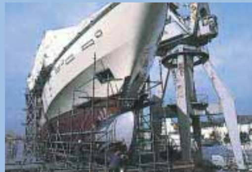
Addition of bulbous bow greatly improved the ride and sea keeping qualities of this 48meter steel motor yacht.
