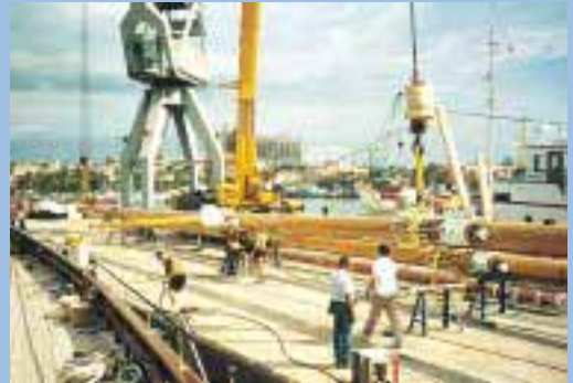
Rigs, both high-tec and classic, are continually serviced in our designated area, including annual checks, painting, modification and even complete rig replacement.
